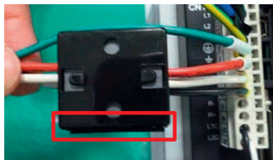
Fig. 5.8 Ferrite ring type KCF-130-B, clips
