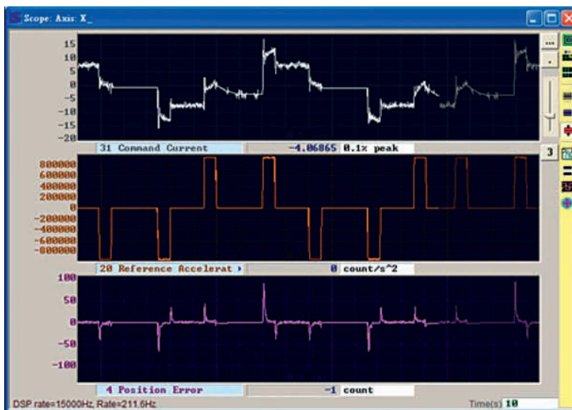
Fig. 7.29 “Scope” for determining the acceleration feedforward
