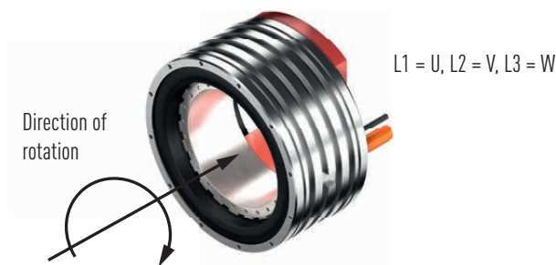
Fig. 5.9 Illustration of rotational direction of the rotor
